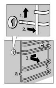
The rails can be removed for cleaning.
